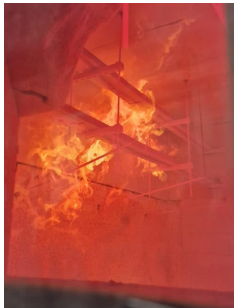
Figure 12 – Internal view of the furnace during the test.
