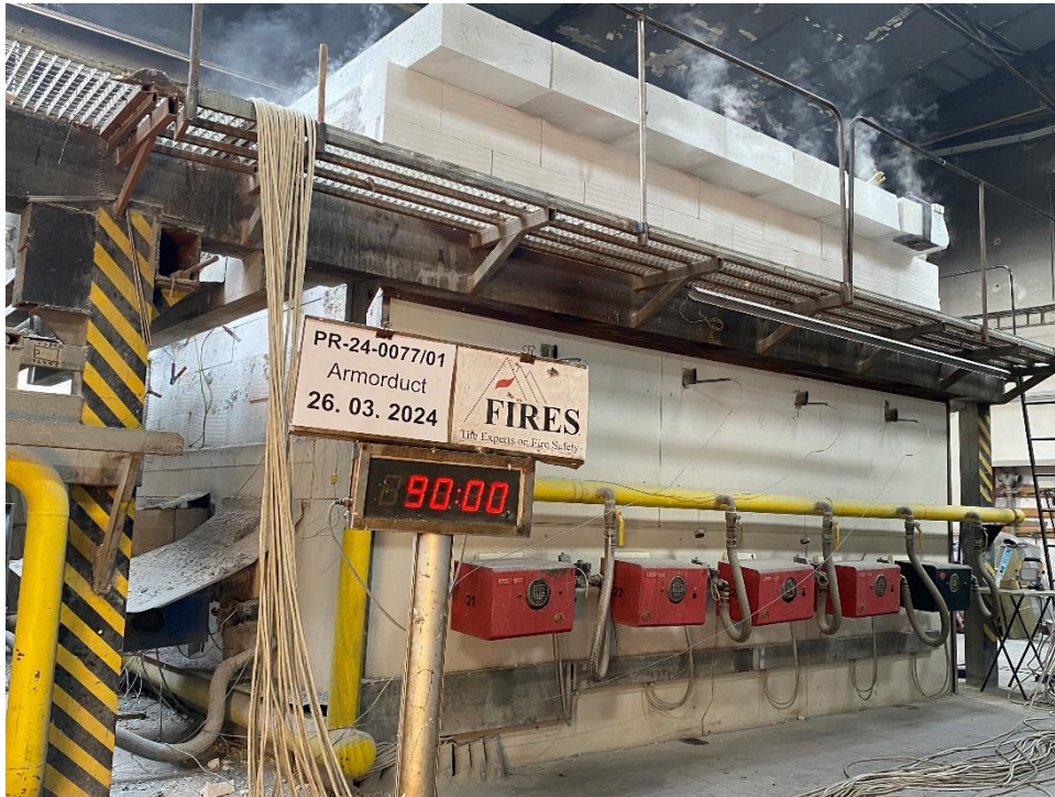
Figure 13 – External view of the furnace at the 90 minute mark.
