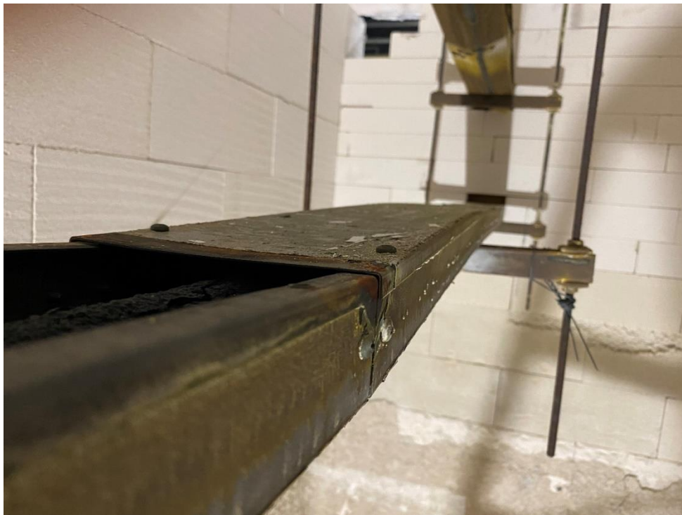
Figure 15 – Armorduct IP4x Cable Trunking after 120 minutes of testing with the cover removed for inspection of the cables.
