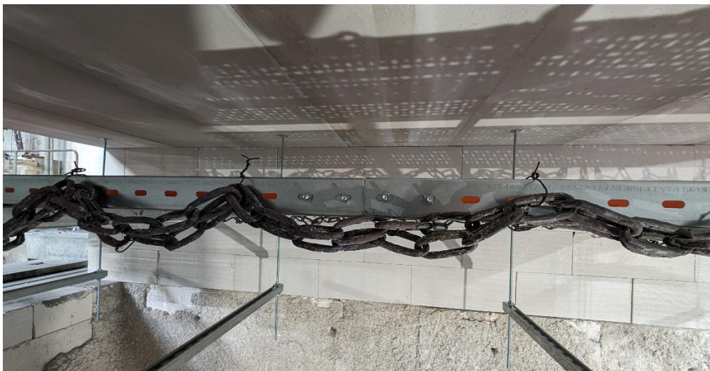
Figure 8 – Armorduct Cable Tray with additional load applied in the form of chains to meet the maximum load of 10kg/m in accordance with DIN 4102-12.
